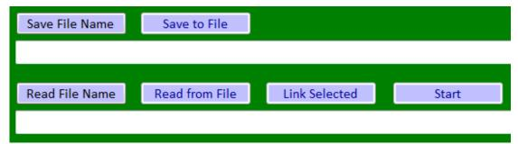
4, The 2 buttons "Save File Name" and "Save to File" are used to save the current work settings to a file including the IP addresses and the % power output of each linked device.
