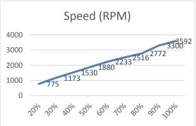
Current consumption and rotation speed varies because of AC adaptor voltage drift and device precision inside the control box. Therefore, +-15% is possible.
