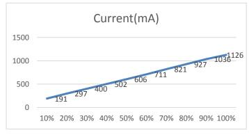
Current consumption varies because of AC adaptor voltage drift and device precision inside the control box. Therefore, +-15% is possible.
